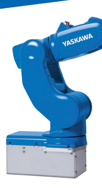
The MotoMINI 6-axis robot was especially designed for handling and assembly of small work pieces. It reduces the size of your production line and helps to increase productivity.
